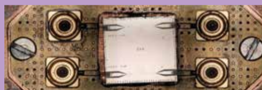
Image of a superconducting quantum chip based on graphene Image credit: F. E. Schmidt
