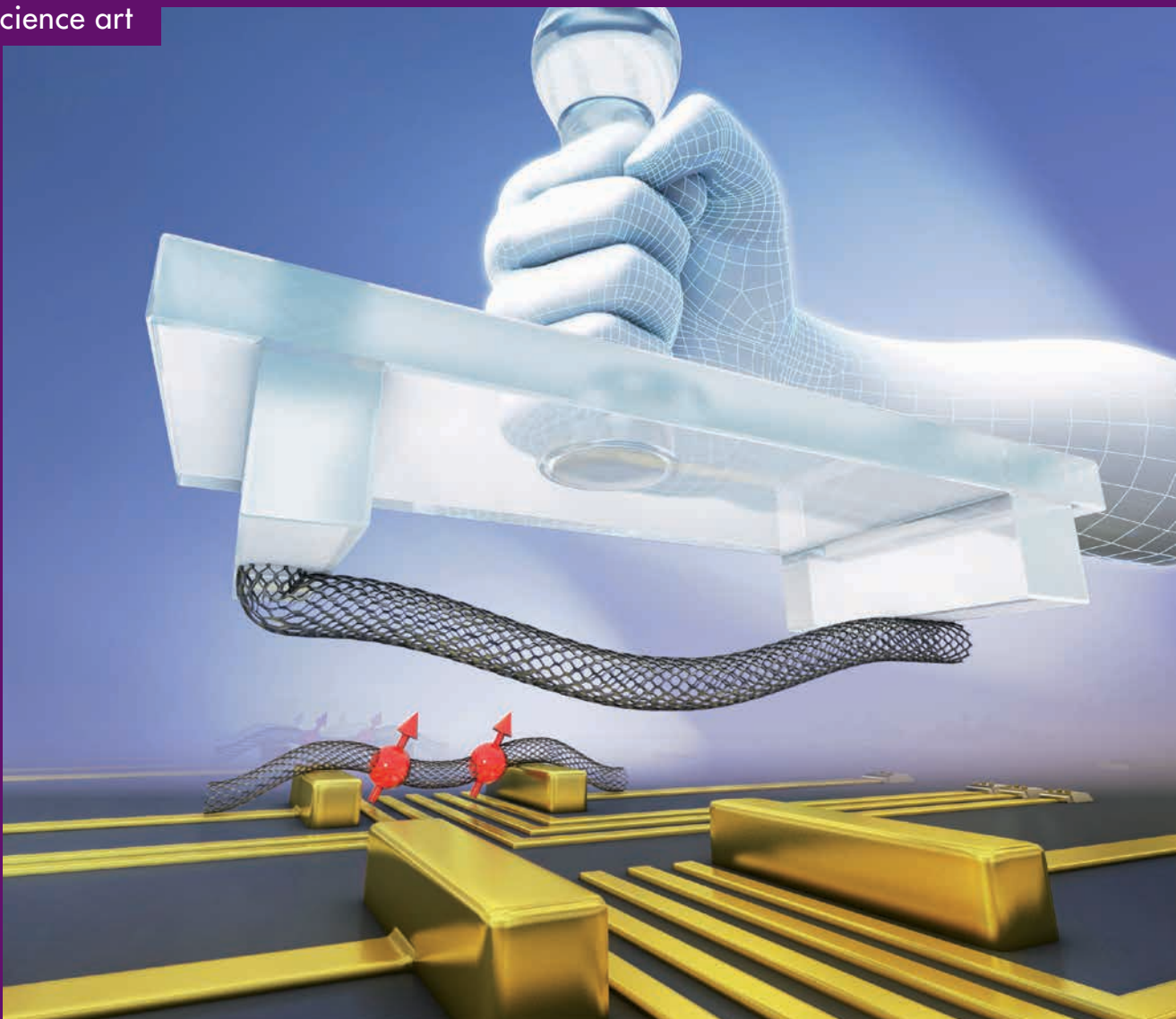
Artist impression of stamping a carbon nanotube. The researchers ‘stamped’ one individual carbon nanotube from the (transparent) growth chip onto the bottom chip (with golden electrodes). The resulting bend in the ultra-clean nanotube allowed the researchers to manipulate single electron spins. Credit: Fei Pei, Edward Laird, Gary Steele, Leo Kouwenhoven Nature Nanotechnology 7, 630-634 (2012). Artist impression made by Fei Pei and Avalon designs.
